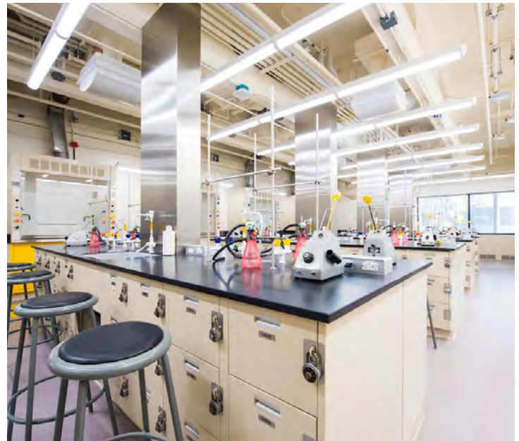
Chemistry Lab, UofA - Teaching laboratory with lockable storage and exposed ceiling for easy access to services
