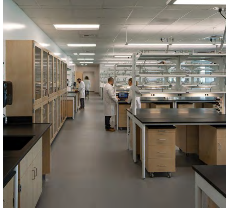
Riverside , UC - Standardized workstations, perimeter casework, mobile casework and ceiling based service distribution
