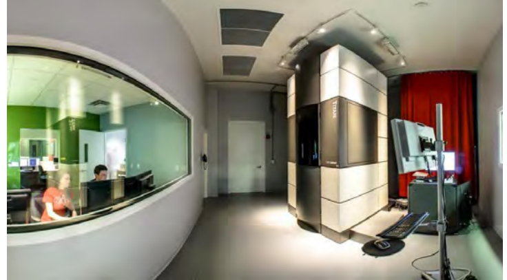
Center for Electron Microscopy and Analysis (CEMAS), Ohio State - Instrument and control room with clear views between for control purposes
