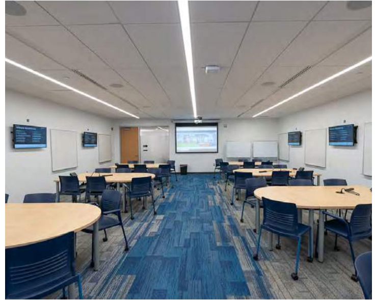
Biological Sciences 1012, UBC - Media sharable learning space with CT flooring, ACT ceiling, and Typ. walls
