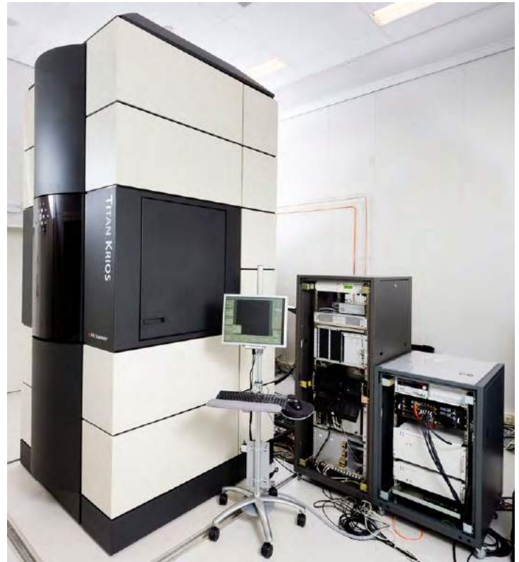
Cryo-electron Microscopy Lab, NeCEN - Instrument room with vibration isolation in slab
