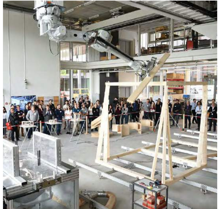
Arch Tec Lab, ETH Zurich - Demonstration of gantry mounted robot arm
