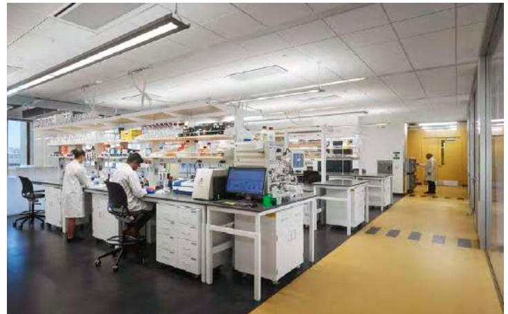
Biodesign Institute, ASU - Flexible wet lab with non-fixed casework and high transparency
